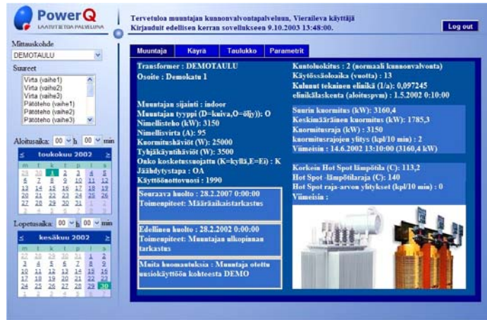
Fig. 2 Condition monitoring information from transformer condition monitoring application
