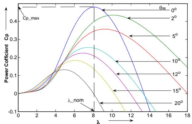
Fig. 1.  $C_p$ - $\lambda$  characteristics.
