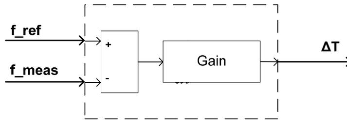
Fig. 7. Proportional controller in supplementary control loop.
