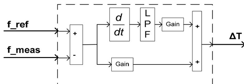
Fig. 6. Proportional plus derivative controller in supplementary control loop.
