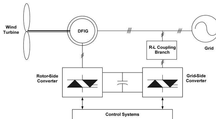
**Fig. 2. The basic configuration of DFIG.**
