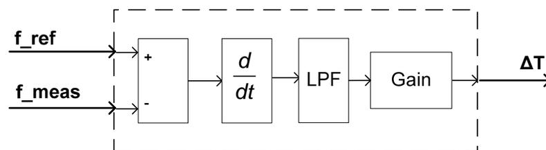
Fig. 5. Derivative controller in supplementary control loop.
