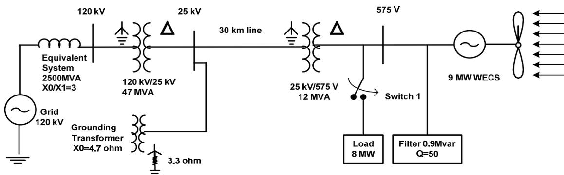
Fig. 8. Single line diagram of 9 MW VS-WT equipped with DFIG.
