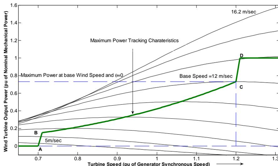
**Fig. 3. The turbine power characteristics.**
