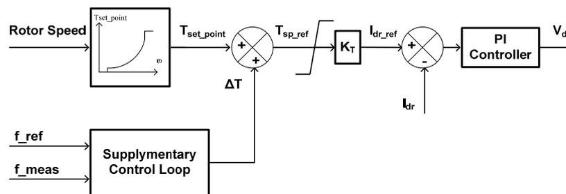
Fig. 4. Supplementary controller for inertia response.
