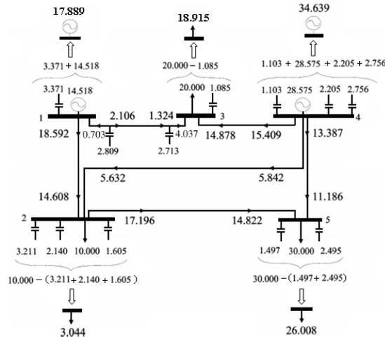
Fig. 6. Reactive power flows in megavolt ampere reactive after introducing the equivalent model line.
