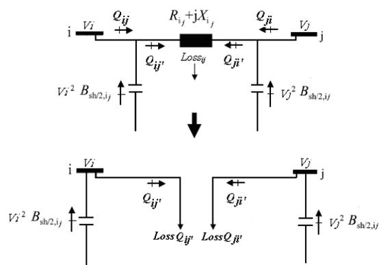
Fig. 3. Equivalent model type 3.
