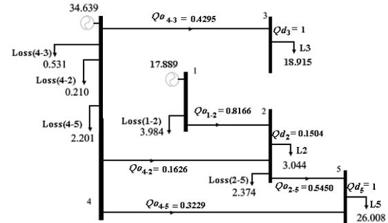
Fig. 8. Model of test system after applied PTM.
