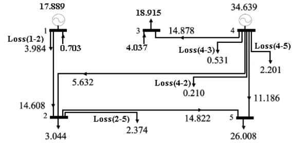
Fig. 7. Lossless system with attributed losses to the sending end of each line.
