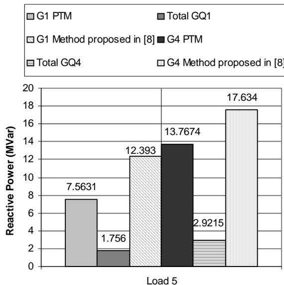
**Fig. 9. Reactive power contribution by each generator to load 5 in MVar.**
