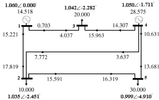
Fig. 5. Five-bus test system with nodal voltages and the reactive power flows in megavolt ampere reactive.
