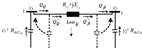
Fig. 1. Equivalent model of the line  $i-j$  (type 1).
