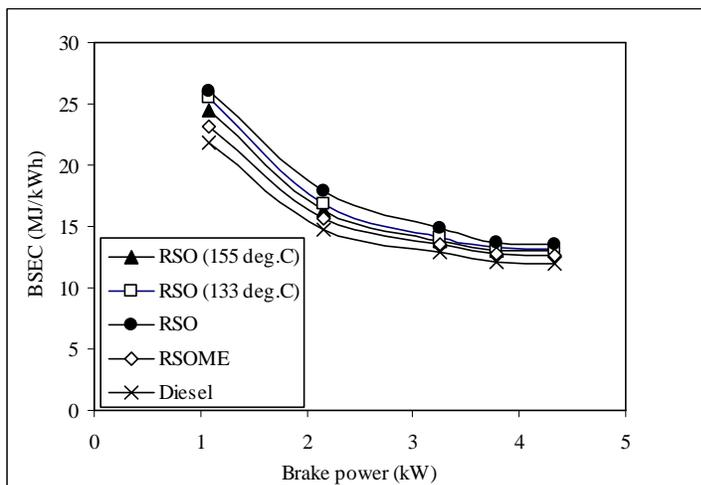
**Fig. 4. Variation of brake specific energy consumption with brake power.**
