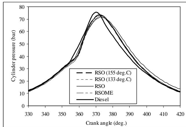
Fig. 10. Variation of cylinder pressure with crank angle.
