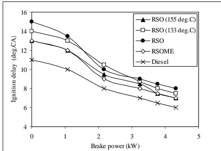
Fig. 14. Variation of ignition delay with brake power.
