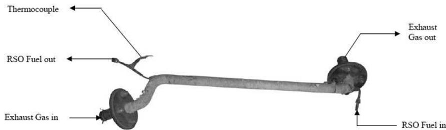
Fig. 1. Photographic view of exhaust gas heat exchanger.
