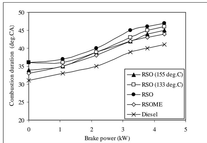
Fig. 15. Variation of combustion duration with brake power.
