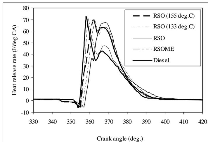
Fig. 13. Variation of heat release rate with crank angle at full load.
