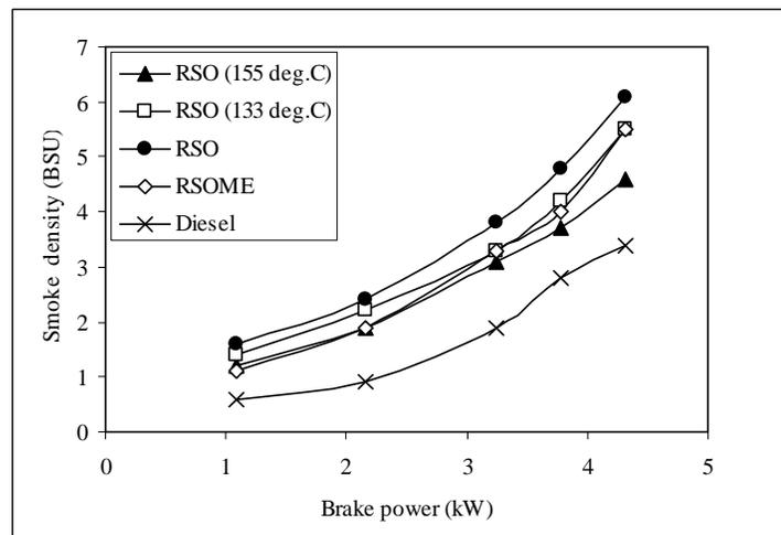
Fig. 6. Variation of smoke density with brake power.
