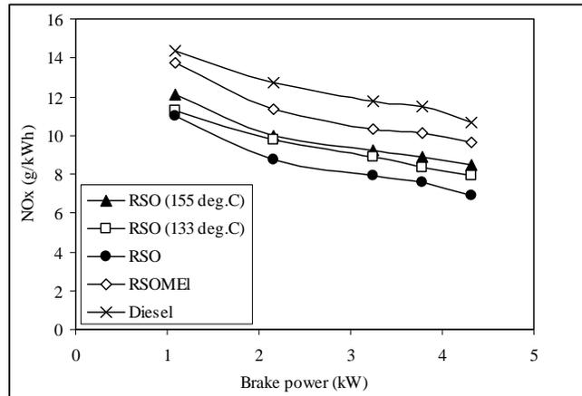
Fig. 9. Variation of nitrogen oxides emission with brake power.
