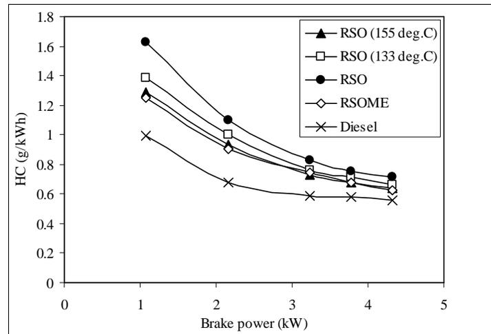
Fig. 8. Variation of hydrocarbon emission with brake power.
