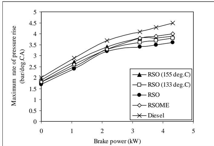
Fig. 12. Variation of maximum rate of pressure rise with crank angle.
