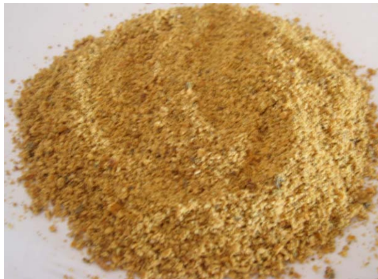
Fig. 2. Powdered OCHF (feed material for biogas production).
