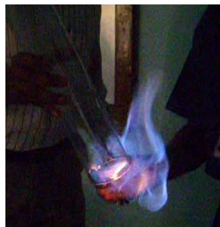
Fig.7. Combustible biogas produced from OCHF.
