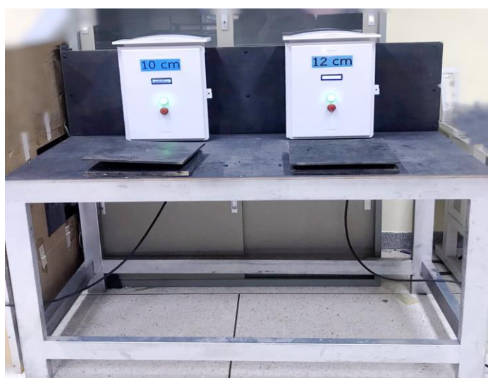
Fig. 4. Physical prototype of the weighing system for 10 cm and 12 cm briquettes.
