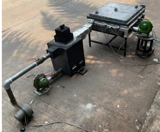
Fig. 1. Experimental setup integrating the downdraft gasifier (black reactor on the left) with the shell-and-tube heat exchanger (steel box on the right).
