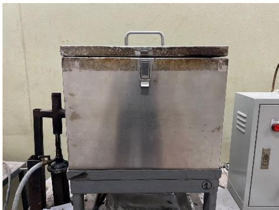
Fig. 3. Torrefaction reactor for the torrefaction process.
