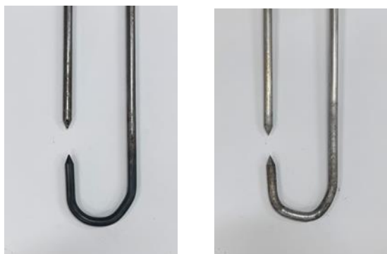
Fig. 7. Electrodes from iron and Al after the experiments.
