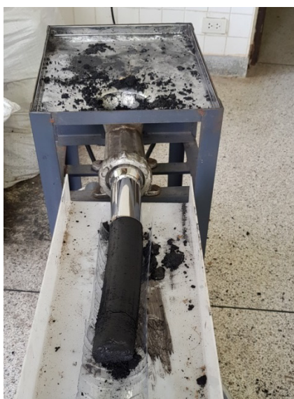
Fig. 2. The charcoal briquettes from a screw press briquette with motor.
