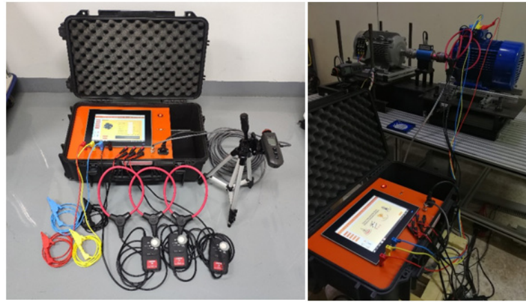
Fig. 4. The non-invasive on-service portable instrument for motor efficiency estimation using the proposed NIECM.
