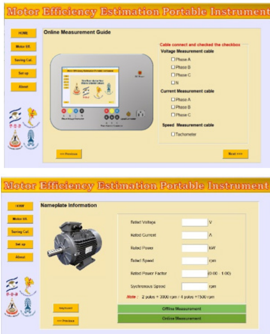
Fig. 5. User interface window of the non-invasive on-service portable instrument for motor efficiency estimation using the proposed NIECM.
