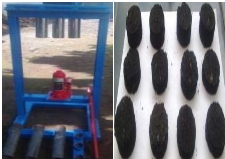
Fig. 2. Briquette presses and products.
