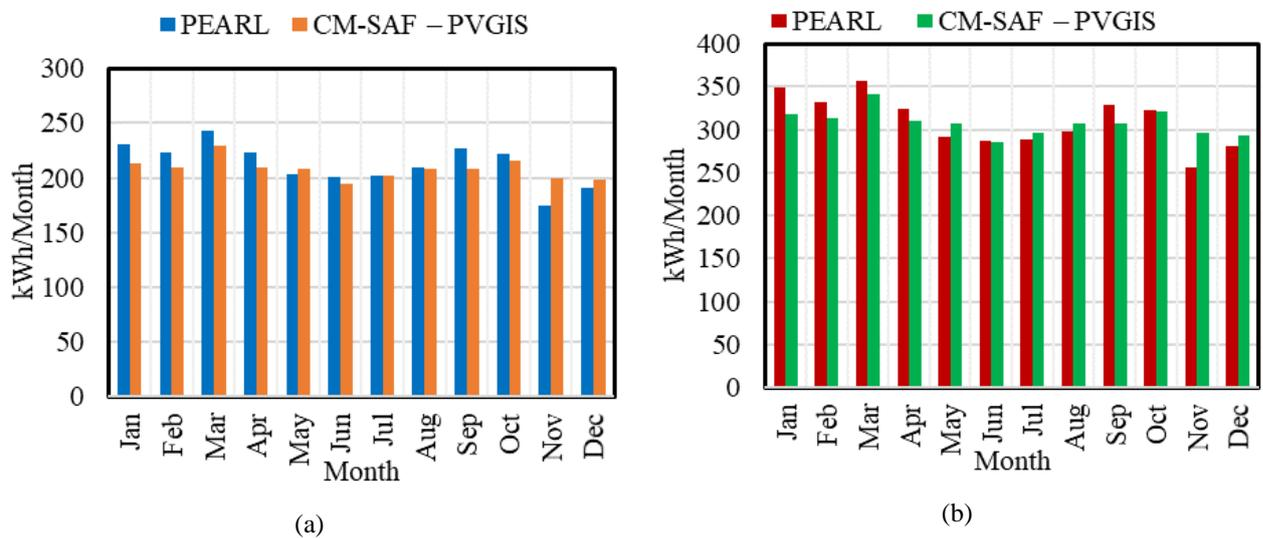
Fig. 4. Average monthly energy generation, (a) polycrystalline solar technology, (b) thin-film solar technology.
