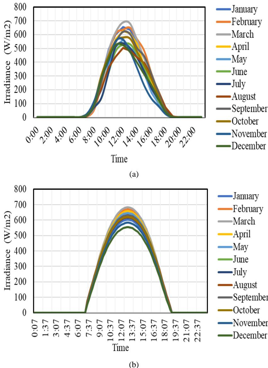
Fig. 3. Average hourly global horizontal solar irradiance at PEARL PV plant, (a) measured, (b) estimated from CM-SAF - PVGIS database.
