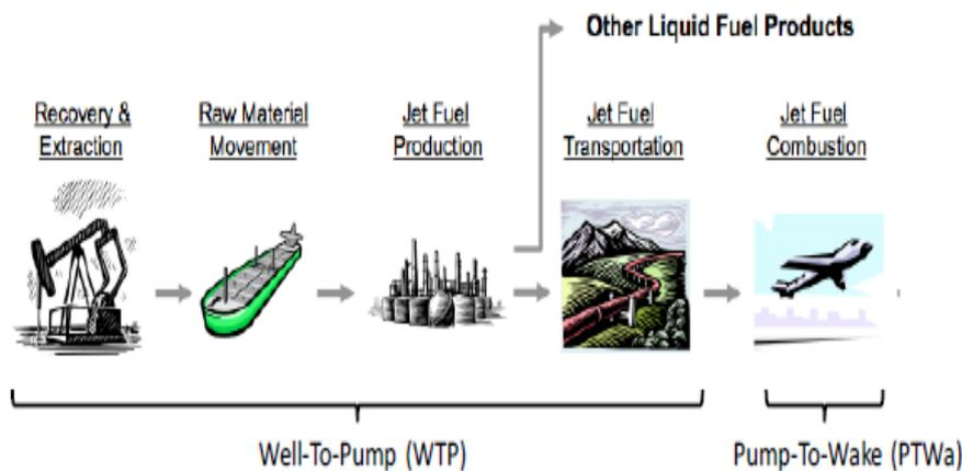
Fig. 1. Well-to-wake lifecycle for conventional fueled aircraft. Source: [9]
