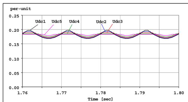
Fig. 23 Capacitor voltages during absorbing reactive power.
