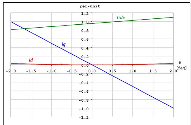
Fig. 3. Steady state characteristic of the STATCOM.
