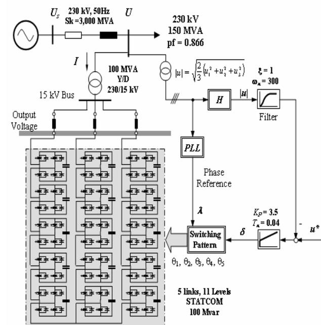
**Fig. 8. The diagram of 230 kV system with short circuit rating of 3000 MVA with voltage regulation by STATCOM.**
