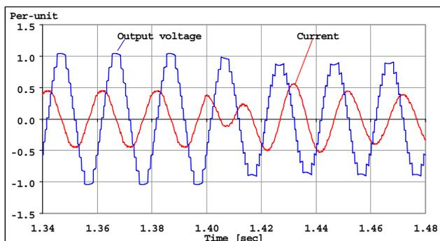
Fig. 19. Output voltage and current waveform of the STATCOM during Event 2.
