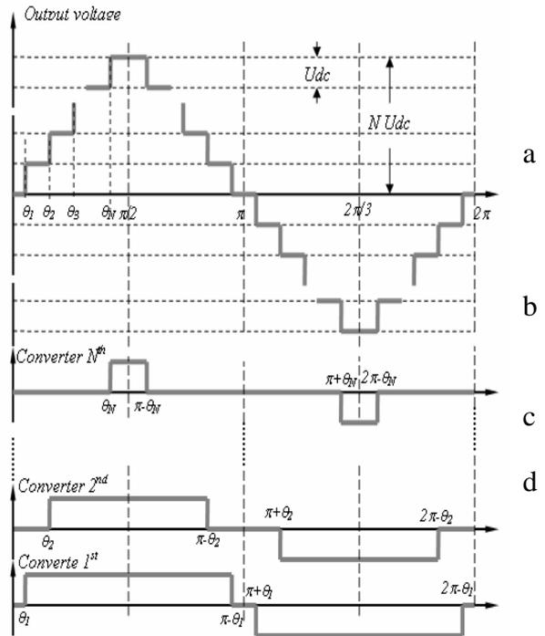
**Fig. 5 Output voltage waveform of a Cascaded  $N$ -level STATCOM (a) and the voltage waveform of individual inverter (b,c, and d).**
