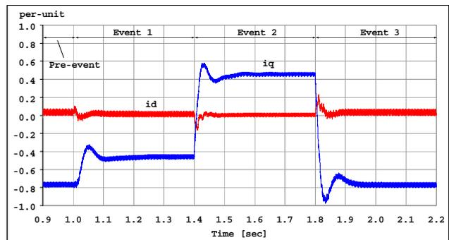
**Fig. 17. Active current (id) and reactive current (iq) of the STATCOM.**
