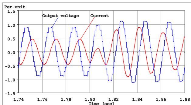
Fig. 20 Output voltage and current waveform of the STATCOM during Event 3.
