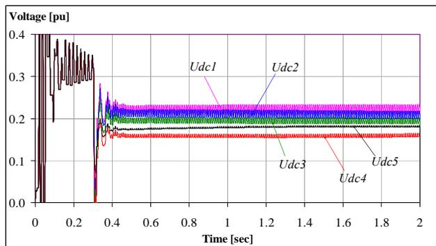
Fig. 10. DC capacitor voltage of each converter when startup from equal DC voltage.
