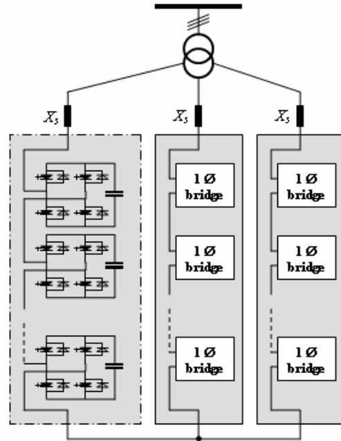
**Fig. 4. Wye connected cascaded multilevel STATCOM.**
