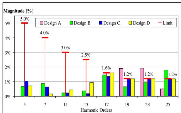
**Fig. 6. Odd harmonic content of the output waveform from Design A to D and harmonic voltage limits from IEC 61000-3-6.**
