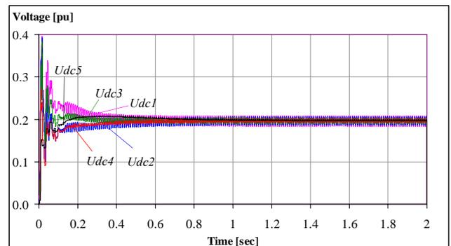
Fig. 12. DC capacitor voltage of each converter during startup.
