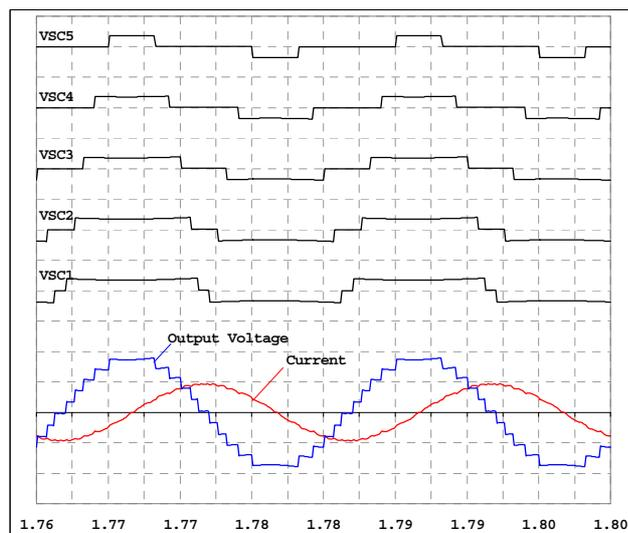
Fig. 21. The output voltage waveform of each H-bridge converter during absorbing reactive power.
