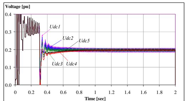
Fig. 13. DC capacitor voltage of each converter when startup from equal DC voltage.
