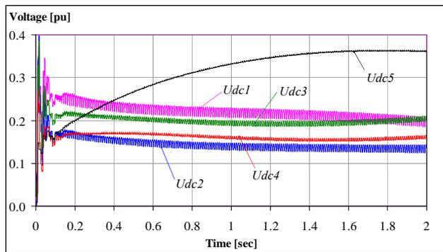
Fig. 9. DC capacitor voltage of each converter during startup.
