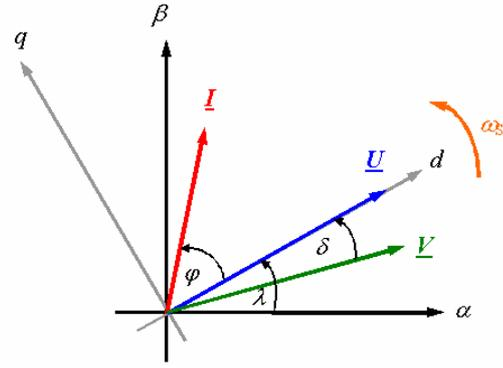
**Fig. 2.** Space vector diagram of voltages and current in synchronously rotating reference frame ( $dq$ ) and stationary reference frame ( $\alpha\beta$ ).
