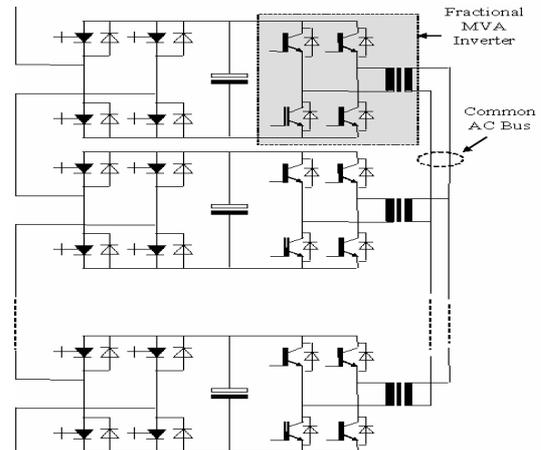
Fig. 11. Auxiliary inverters and a common AC Bus.
