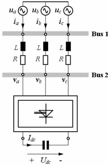
**Fig. 1.** An equivalent circuit of a simple two bus power system with a STATCOM circuit.
