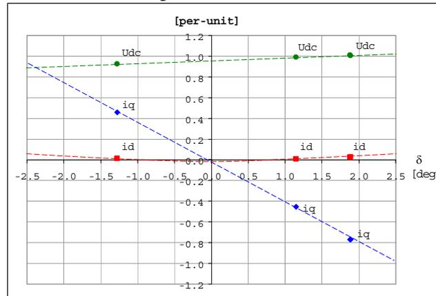
Fig. 26. Steady state performance of the STATCOM.
