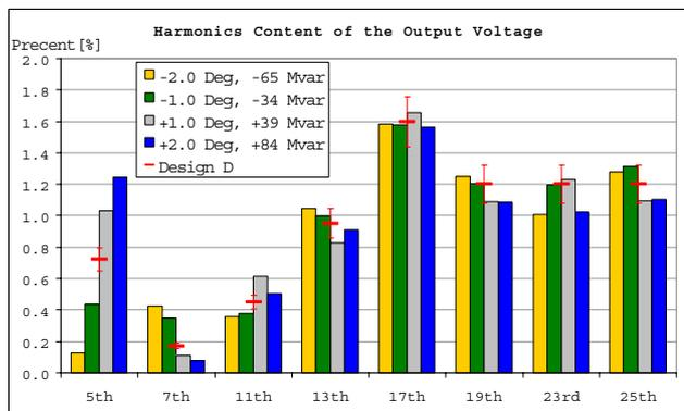
Fig. 25. Spectrum of 5<sup>th</sup> 7<sup>th</sup> 11<sup>th</sup> 13<sup>th</sup> 17<sup>th</sup> 19<sup>th</sup> 23<sup>rd</sup> 25<sup>th</sup> harmonics content of the output voltage waveform with ripples in the capacitor voltage.
