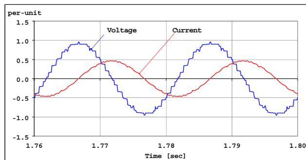
Fig. 22. The voltage and current waveforms of the secondary winding (15 kV bus) during absorbing reactive power.
