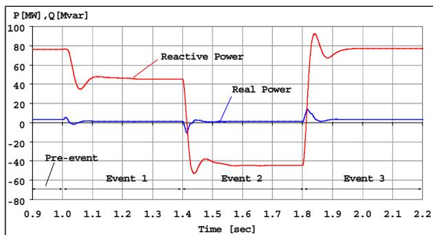
**Fig. 16. Real and reactive power of the STATCOM.**
