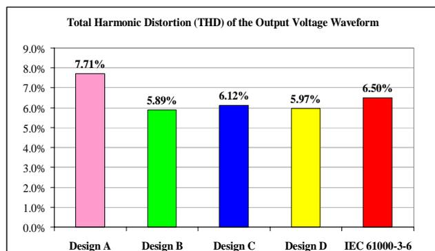
**Fig. 7. Comparison of THD from Design A to D and THD limit from IEC 61000-3-6.**
