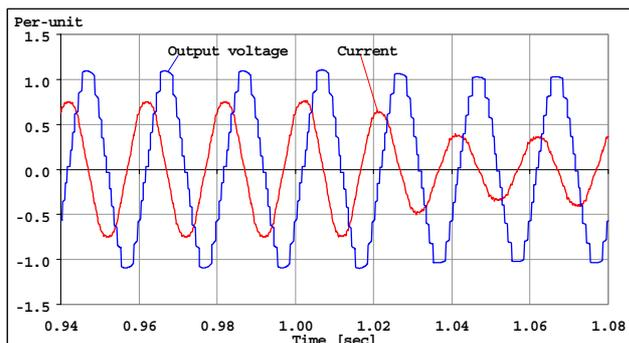
Fig. 18. Output voltage and current waveform of the STATCOM during Event 1.
