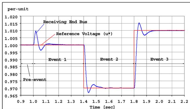
**Fig. 14. Receiving end voltage and Reference Voltage**
