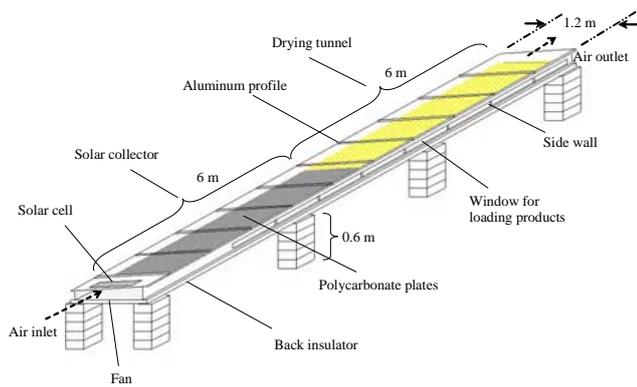
**Fig. 1. Schematic diagram of the solar tunnel dryer with polycarbonate cover.**
