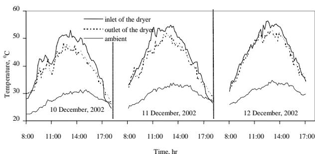
Fig. 8. Variation of the temperatures of the air at the inlet and outlet of the dryer and the ambient air in the course of the drying.
