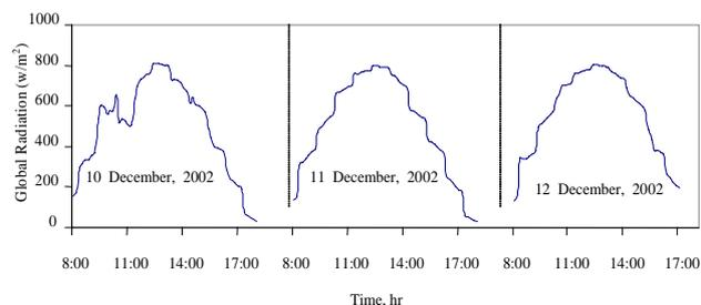
Fig. 7. Variation of global solar radiation in the course of the drying.
