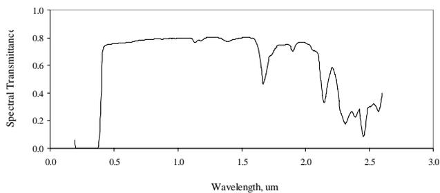
**Fig. 2. Spectral transmittance of the polycarbonate plate.**
