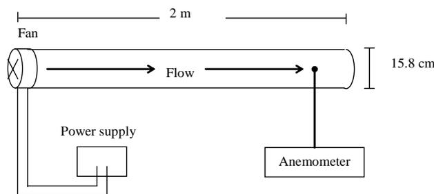
**Fig. 3. Schematic diagram of the equipment for determining the relation between the air flow rate and the power required by dc-axial flow fan.**
