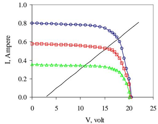
**Fig. 4. Experimental I-V curves of the solar cell module and the dc-axial flow fan.**
