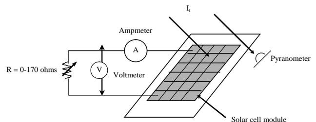
**Fig. 6. Schematic diagram of equipment for determining characteristic curves of the solar cell module.**
