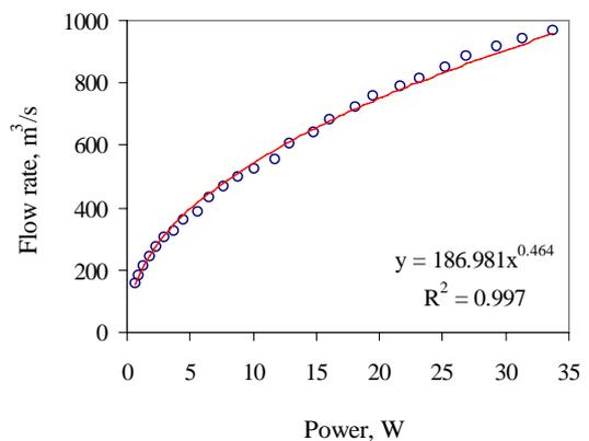
**Fig. 5. Relation between the air flow rate and power required by the dc-axial flow fan.**
