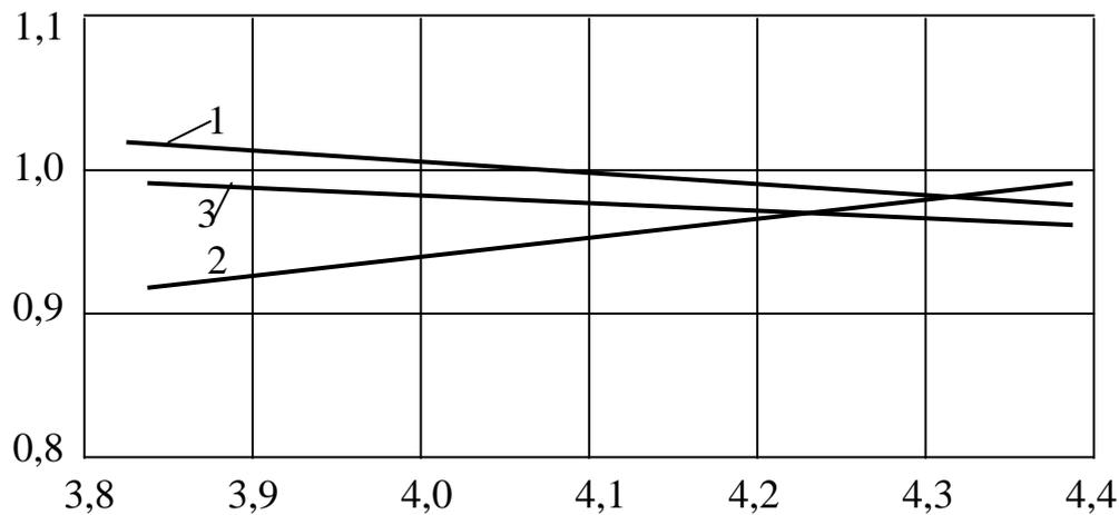
X axis – logarithm of Reynolds number; Y axis – relation of  $N_{ui}/Nu$ . Legend: 1 – with panel, 2 – half tubes, 3 –  $\Gamma$ -shaped panels.
