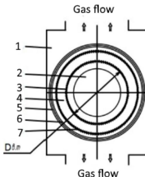
1 – exhaust gases duct, 2 – furnace, 3 – internal cylindrical membrane type furnace screen, 4 – behind-the-screen gas pass, 5 – external heat insulated panels, 6 – heat reflecting panels, 7 – coaxial external furnace screen
