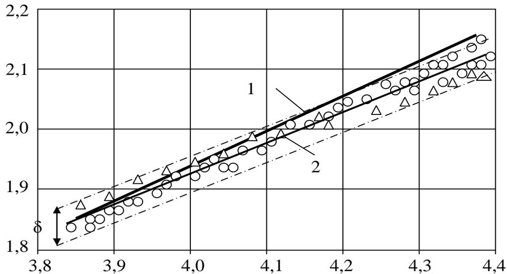
X axis – logarithm of Reynolds number; Y axis – logarithm of Nusselt number. Legend: 1 – tube column classic alternate arrangement  $Nu = 0,35 \times Re^{0,6}$  [12], 2 – dependency obtained experimentally with three types of swirler devices ( $\delta$  – inaccuracy).
