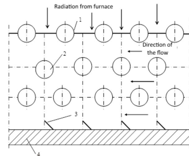
1 – all-welded membrane panel, 2 – tube column with alternate arrangement, 3 – bent panels, 4 – portable heat isolated panel.
