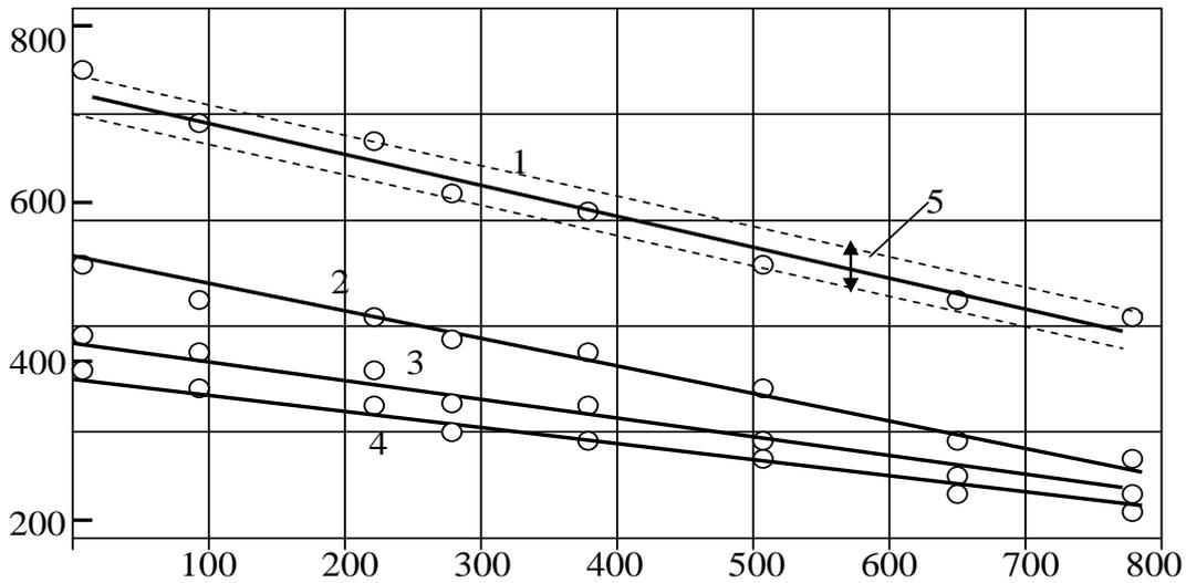
X axis – length of a channel, mm; Y axis – static pressure, Pa. Legend: 1 – Re number = 21500; 2 – Re number = 17000; 3 – Re number = 15500; 4 – Re number = 14000; 5 – experimental inaccuracy.
