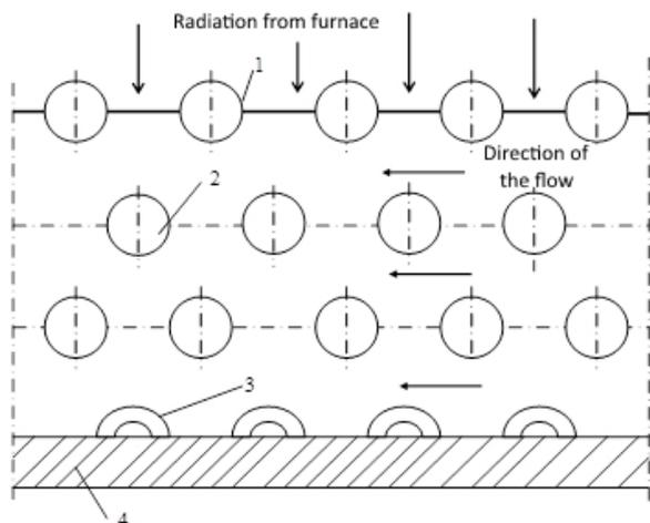
1 – all-welded membrane panel, 2 – tube column with alternate arrangement, 3 – swirler devices in the form of half tubes, 4 – portable heat isolated panel.
