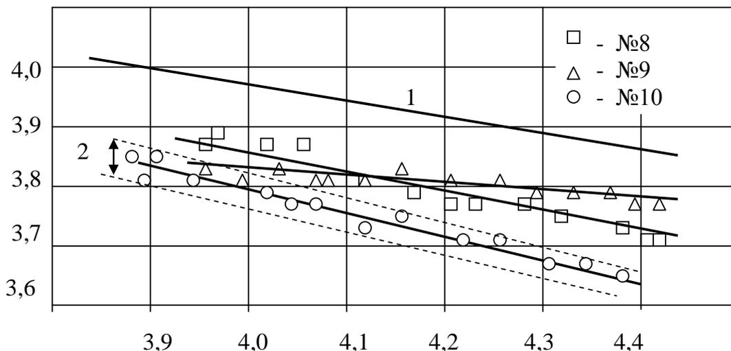
X axis – Artificial number of Reynolds number; Y axis – artificial number of  $(1000\xi)$ . Legend: 1 – normative tube column with alternate arrangement, 2 – precision of generalization; №8 – with half cylindrical rails; №9 – with panel rails; №10 – panel with bent edge.
