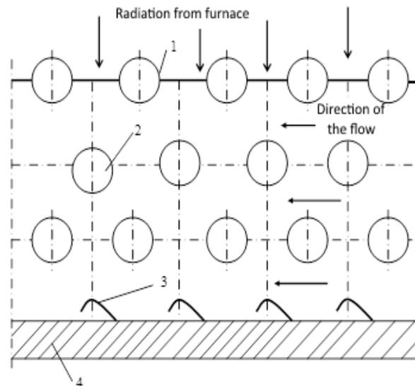
1 – all-welded membrane panel, 2 – tube column with alternate arrangement, 3 – Γ-shaped panels, 4 – portable heat isolated panel.
