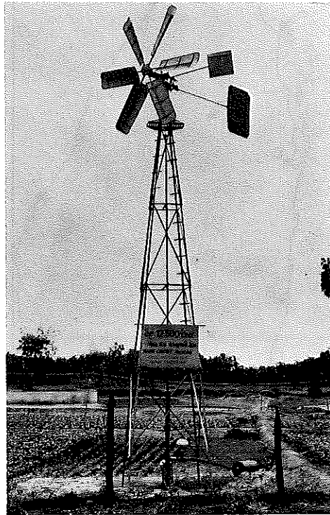
Fig. 9 The WEU windmill water pump (5 m diameter rotor)
