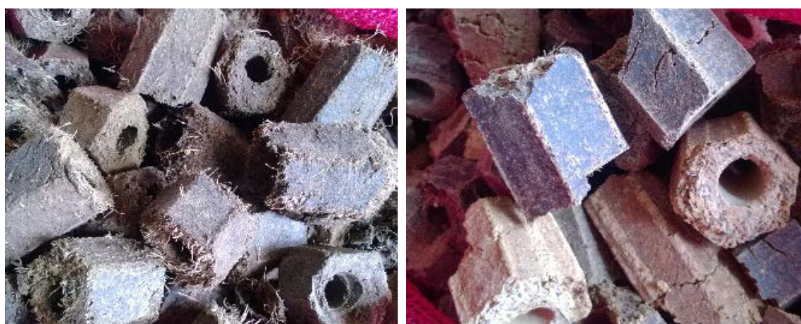
Fig. 4. Biomass briquetted from a.) Oil palm wastes b.) Tung oil tree wastes.
