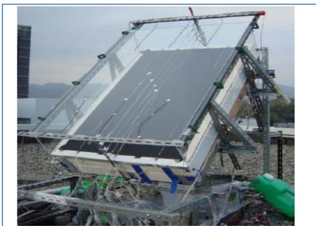
Fig. 29. Photograph of the prototype solar chimney with PCM modules for natural ventilation [44].
