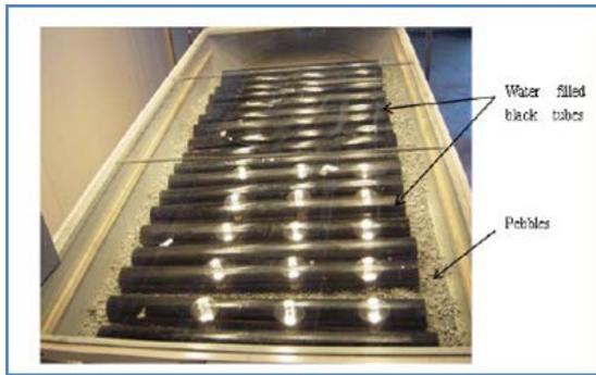
**Fig. 19. The solar collector layout [31].**
