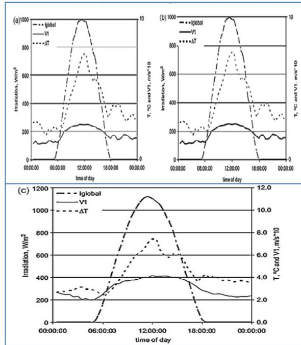
Fig. 11. An average of measured solar radiation, temperature and velocity. (a) For selected 5 clear days of October (with turbine installed), (b) for selected 6 clear days between 19 and 30 October (with turbine removed), (c) for 6 days between 14 and 21 November (with turbine and diffuser removed) [17].
