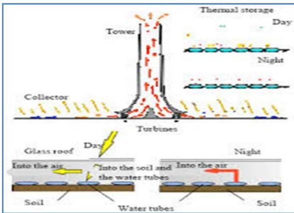
**Fig. 13. Heat storage underneath of the roof collector using water-filled black tubes [24].**
