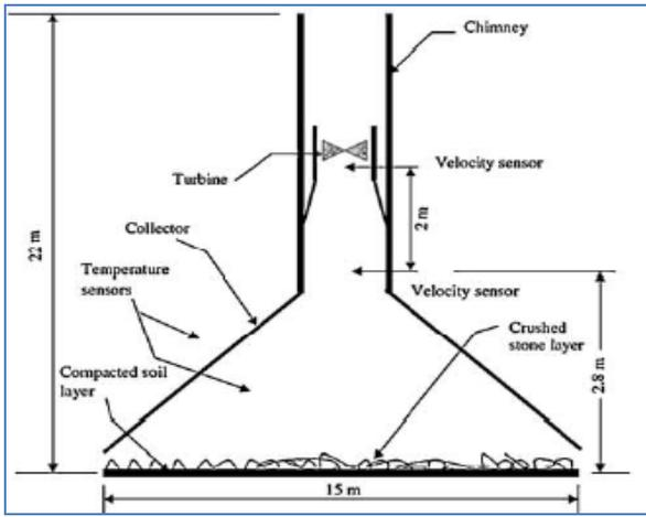
Fig. 10. Schematic overview of the Botswana solar chimney power plant [17].
