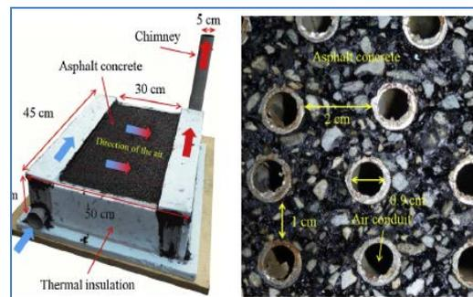
Fig. 12. Detail of the air conduits in the asphalt [21].
