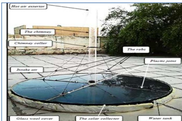
Fig. 25. Photograph of the experimental scale model of the solar chimney power plant by Haider [36].
