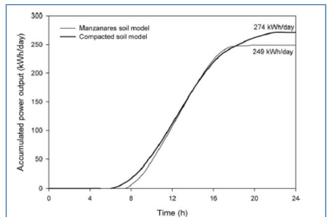
Fig. 9. Numerical investigation on the soil compaction influence. Accumulated power output [16].
