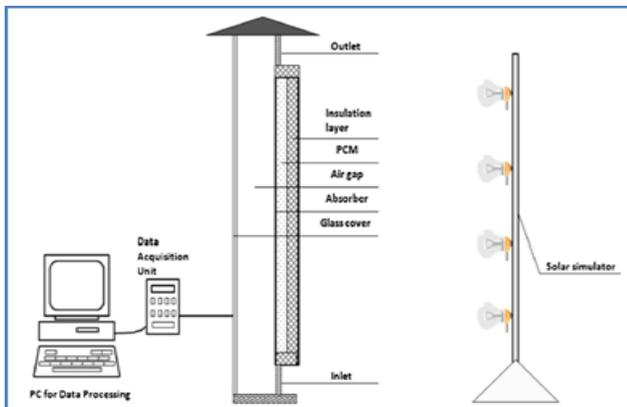
Fig. 27. Schematic of the experimental solar chimney system (closed model) [40],[ 41].
