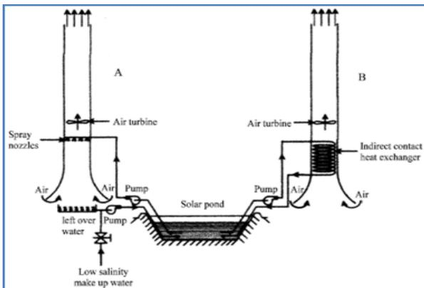
Fig. 16. Concepts for combining a chimney with a solar pond to generate power [28].
