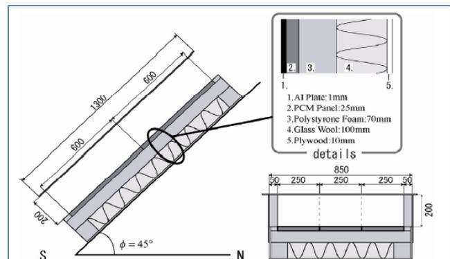
Fig. 30. Cross-sectional view of chimney with built – in PCM storage [44].
