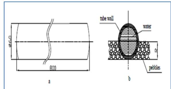
**Fig. 20. Profile chart of thermal storage in the solar collector [31], (a) The dimension of water tube for thermal storage material, (b) Cross- section of water in radial.**
