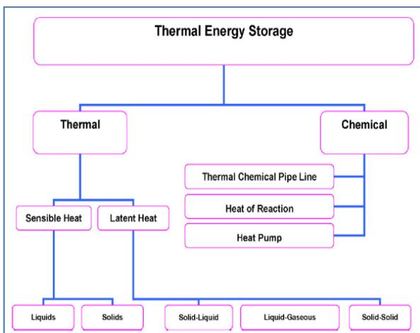
Fig. 3. Different types of thermal storage of solar energy application [37].
