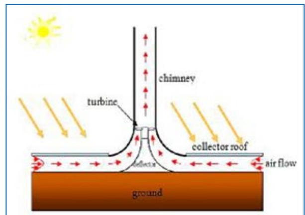
Fig. 1. Schematic diagram of solar chimney [1].
