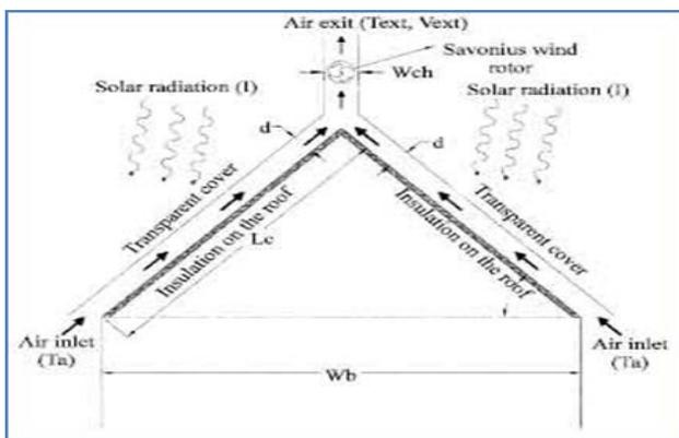
Fig. 23. Schematic of roof- top solar chimney [34].
