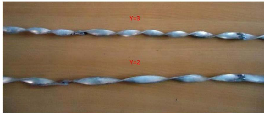
Fig. 2. (a) Plain Twisted Tapes (P-TT).
