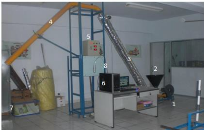
Fig. 1. Experimental set up to measure power requirement of a pneumatic conveyor, and the drying process occurring within the conveyor.
