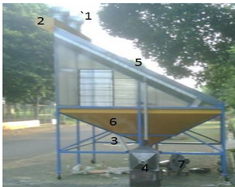
Fig. 1. Schematic diagram of the proposed 2,5 ton maximum capacity 2nd generation of a recirculation type hybrid ICDC solar dryer.
